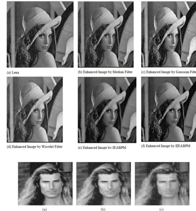
Figure 4: (a) Original 256 \times 256 Fabio image corrupted with Gaussian noise and its reconstruction from 20% randomly-selected Fourier coefficients using (b) total-variation minimization and (c) \ell_1 -minimization of its bivariate Haar coefficients
